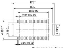
Recommended solder paste thickness: 120  $\mu m$
