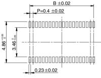
Recommended solder paste thickness: 120  $\mu$ m
