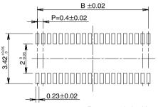
Recommended solder paste thickness: 120  $\mu m$
