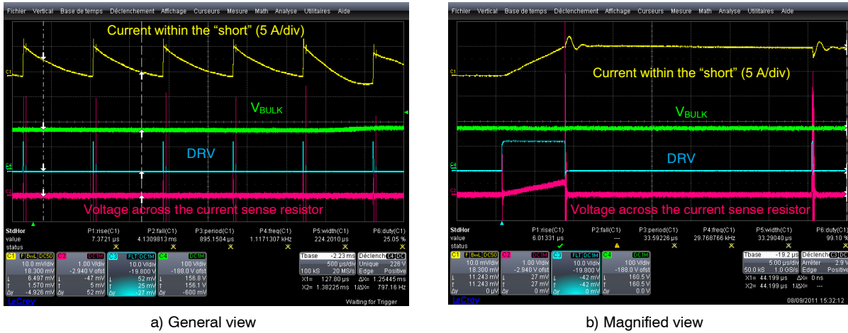
Figure 17. Shorting the Bypass Diode and the NTC
