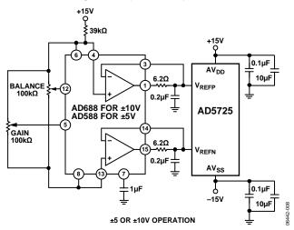
Figure 28. Symmetrical Bipolar Operation
