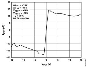
Figure 23. IOUT VS.  $V_{OUT}$  ( $V_{SUPPLY} = \pm 15 V$ )
