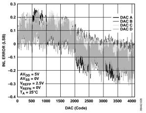
Figure 14. Channel-to-Channel Matching ( $V_{SUPPLY} = +5 V$ )
