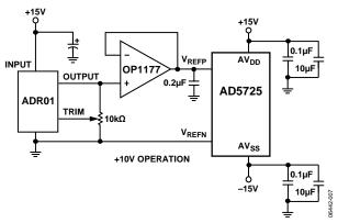
Figure 27. Unipolar +10 V Operation
