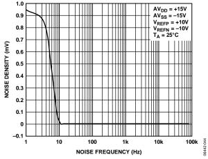
Figure 22. Output Noise Spectral Density vs. Frequency
