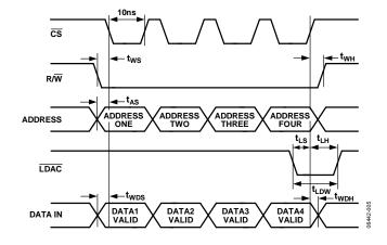
Figure 5. Double Buffer Mode Timing
