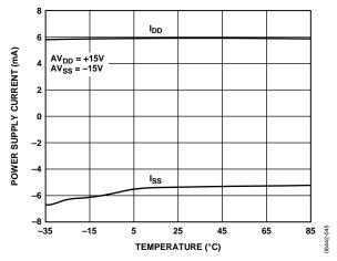
Figure 21. Power Supply Current vs. Temperature
