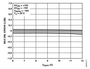
Figure 7. DNL vs.  $V_{REFP}$  ( $V_{SUPPLY} = \pm 15 V$ )
