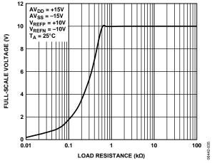
Figure 19. Output Voltage Swing vs. Resistive Load
