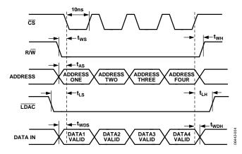
Figure 4. Single Buffer Mode Timing
