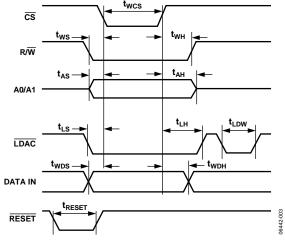
Figure 3. Data Write Timing
