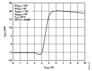
Figure 24. Iout vs.  $V_{OUT}$  ( $V_{SUPPLY} = +15 V$ )
