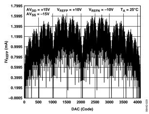
Figure 18. IV<sub>REFP</sub> vs. DAC Code
