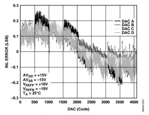
Figure 13. Channel-to-Channel Matching ( $V_{SUPPLY} = \pm 15 V$ )
