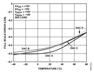
Figure 11. Full-Scale Error vs. Temperature
