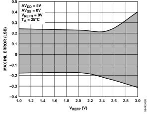
Figure 10. INL vs.  $V_{REFP}$  ( $V_{SUPPLY} = +5 V$ )
