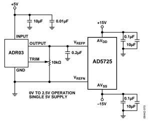
Figure 30. +5 V Single-Supply Operation
