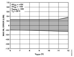
Figure 9. INL vs.  $V_{REFP}$  ( $V_{SUPPLY} = \pm 15 V$ )
