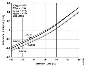
Figure 12. Zero-Scale Error vs. Temperature
