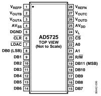
Figure 6. Pin Configuration Diagram
