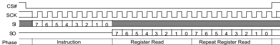
Figure 54. Read Bank Register (BRRD 16h) Command
