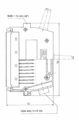
Cable housings KSG 253 for female ribbon-cable (IDC) – connectors type C
