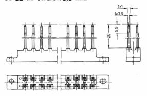
Remaining dimensions as for wiring strip VE 32-ac-1 x 1
