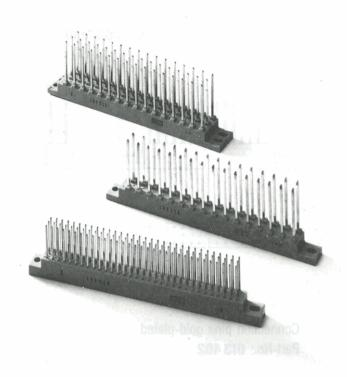
19" subracks have space for mounting female connectors to DIN 41 612 vertically in the wiring plane while the top and bottom edge wiring fields have room for mounting wiring strips and plug-on distribution strips horizontally. These strips are also suitable for mounting in the wiring plane. The wiring strips VE 64 and VE 96 with gold-plated  $0.6 \times 0.6$  mm connection pins on a 2.54 mm grid are suitable for plugging on female connectors type C to DIN 41 612.
