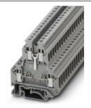
Component terminal block, Connection type: Screw connection, Cross section: 0.2 mm<sup>2</sup> - 4 mm<sup>2</sup>, AWG: 24 - 12, Nominal current: 32 A, Nominal voltage: 500 V, Length: 56 mm, Width: 6.2 mm, Color: gray, Assembly: NS 35/7,5, NS 35/15, NS 32
