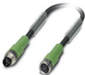
Sensor/actuator cable, 3-position, PUR halogen-free, black-gray RAL 7021, Plug straight M8, on Socket straight M8, cable length: 1 m
