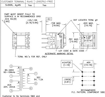
Customer to tie terminals 5&6 and 7&8 on pcb for correct operation.
