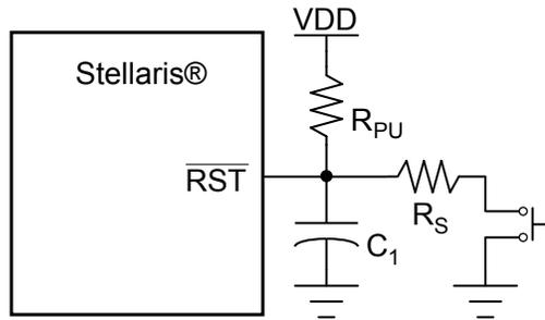
Typical  $R_{PU} = 10 \text{ k}\Omega$
