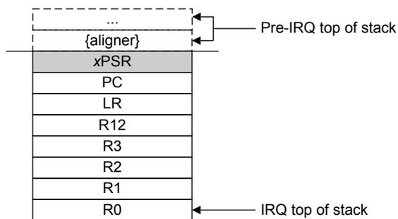
Immediately after stacking, the stack pointer indicates the lowest address in the stack frame. Unless stack alignment is disabled, the stack frame is aligned to a double-word address. If the **STKALIGN** bit of the **Configuration Control (CCR)** register is set, stack align adjustment is performed during stacking.
