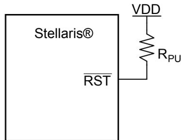
$R_{\text{PU}} = 0$  to 100 k $\Omega$
