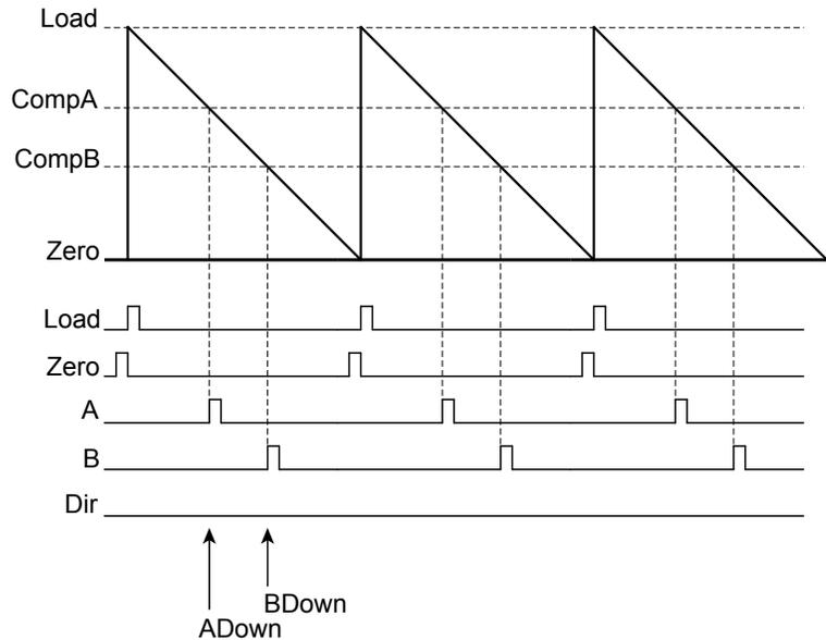
**Figure 14-4. PWM Count-Up/Down Mode**
