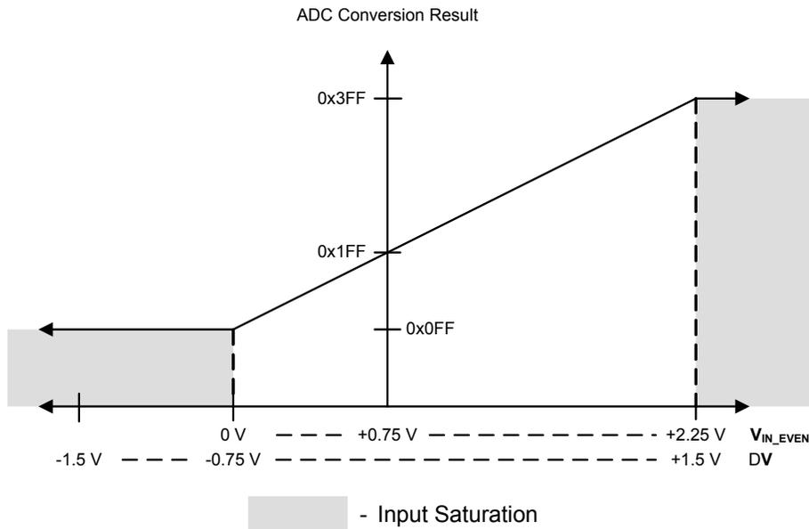
Figure 10-4. Differential Sampling Range,  $V_{IN\_ODD} = 2.25\text{ V}$
