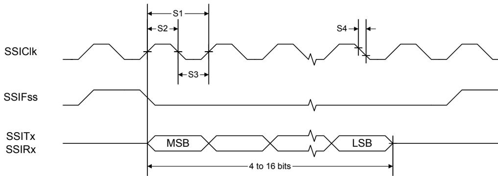
Figure 18-13. SSI Timing for MICROWIRE Frame Format (FRF=10), Single Transfer
