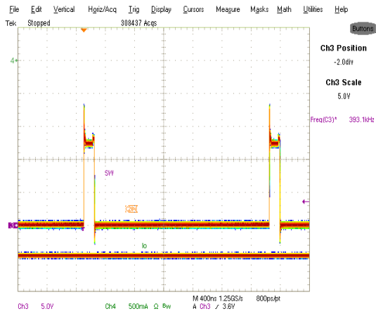
Fig. 19: Inductor node at -3A, sinking current, Ch 3 :SW, Ch 4 :I out
