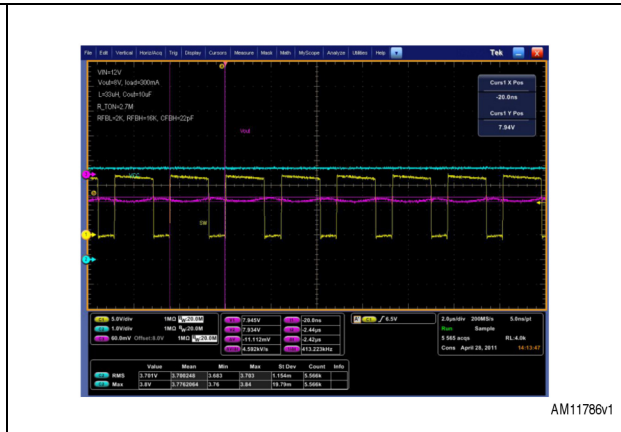
Figure 27. Load = 300 mA. Switching frequency = 410 kHz
