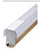
Cover profile, for covering terminal strips, snaps onto cover profile carrier AP 2-TU, can be marked with insert strip AP-ES. Cover profile carriers should be placed at the ends and at intervals of approx. 40 cm. Length: 1 m
