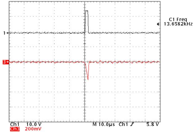
Figure 26. CS Pin at Light Load Condition
