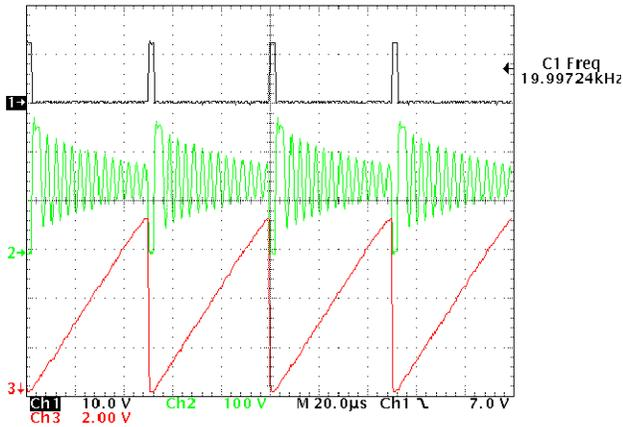
Figure 24. CT and Drain at Light Load
