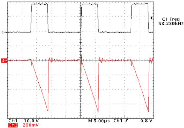
Figure 25. CS Pin at Full Load Condition
