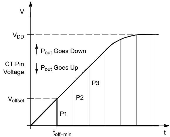
Figure 18. CT Pin Voltage ( $P_{out1} > P_{out2} > P_{out3}$ )
