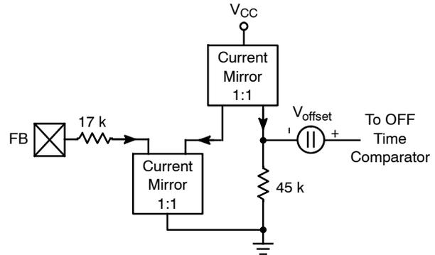
Figure 13. Feedback Loop - OFF Time Control
