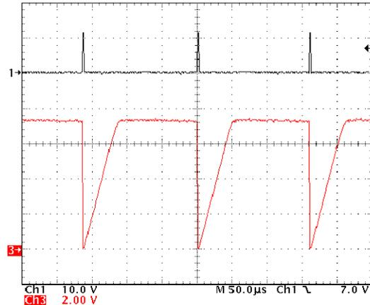
**Figure 23. CT Voltage at No Load Condition**
