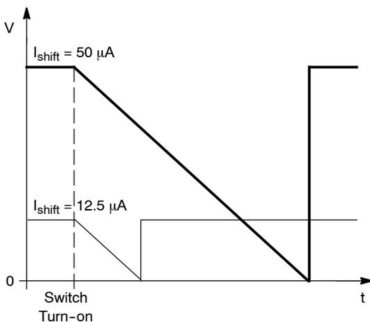
**Figure 20. CS Pin Voltage**
