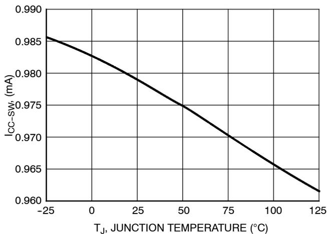
Figure 5. Operating Current Consumption vs. Junction Temperature
