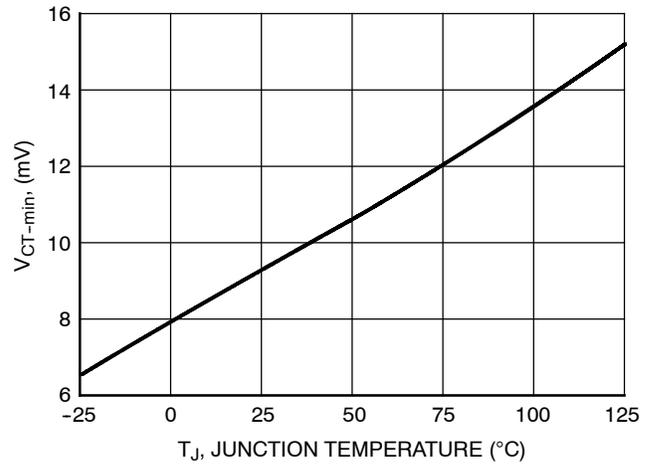
**Figure 10. CT Pin Threshold vs. Junction Temperature**
