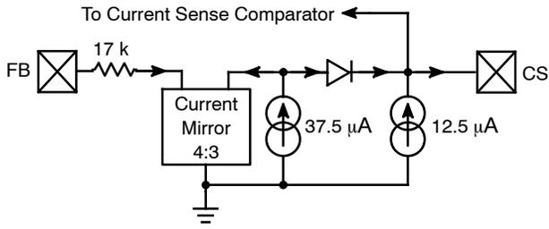
Figure 15. Feedback Loop - Current Sense Control
