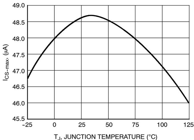
Figure 7. Current Sense Source Current vs. Junction Temperature
