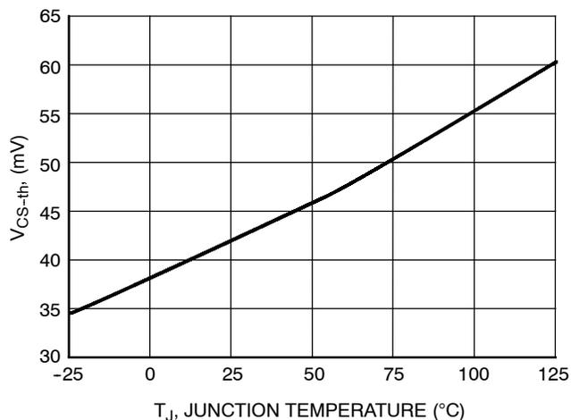
Figure 8. Current Sense Threshold vs. Junction Temperature
