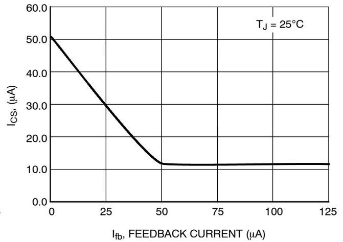
**Figure 12. Current Sense Source Current vs. Feedback Current**
