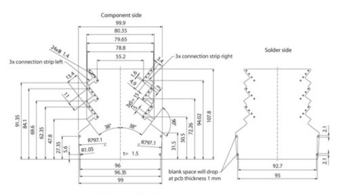
non dimensioned radii max R1 inhibited surface
