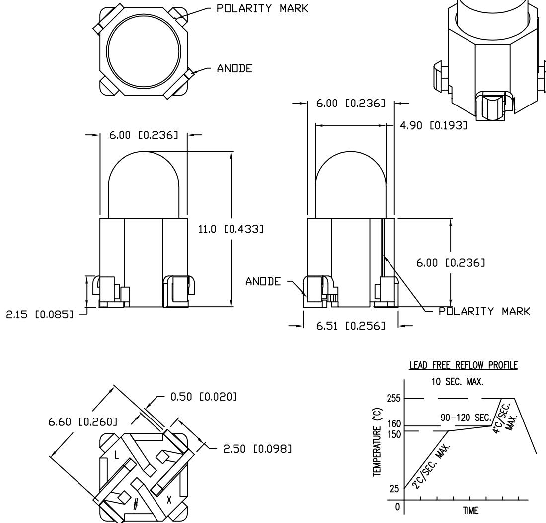
\*UNLESS OTHERWISE SPECIFIED TOLERANCES PER DECIMAL PRECISION ARE: X=±1 ( $\pm 0.039$ ), XX=±0.5 ( $\pm 0.020$ ), XXX=±0.25 ( $\pm 0.010$ ), XXXX=±0.127 ( $\pm 0.005$ ). LEAD SIZE=±0.05 ( $\pm 0.002$ ), LEAD LENGTH=±0.75 ( $\pm 0.030$ ). MIN=+DECIMAL PRECISION MAX=+0.00
