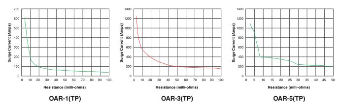
The Surge current charts are approximations of the capabilities of the OAR product and should not be used to the exclusion of actual testing. The relative high surge currents depicted in the charts are as a result of the robust all metal welded construction and the heat carrying capability of metal. Additionally the OAR resistive wire provides large relative cross section for current flow as compared to other resistor technologies, such as thin film, thick film, or metal strip.
