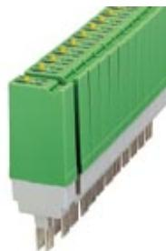
Relay connector, fitted with miniature switching relay, contacts (AgNi): Medium to large loads, 1 N/O contact, 220 V DC input voltage, with light indicator, can be plugged into basic terminal blocks
