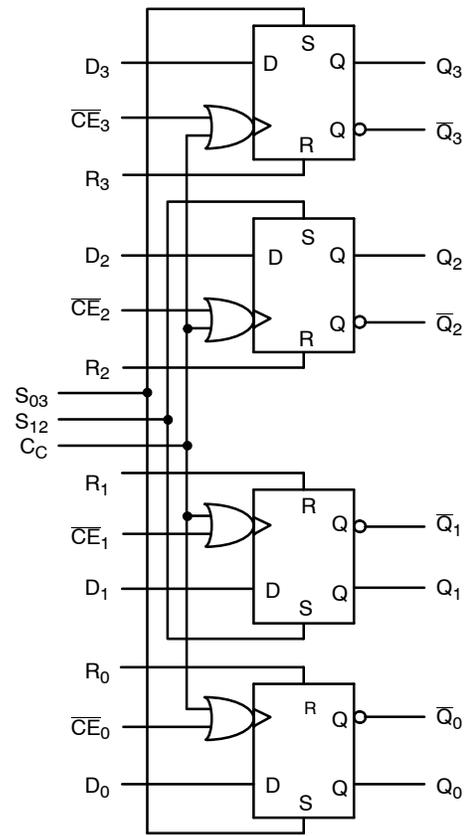
**Figure 2. Logic Diagram**
