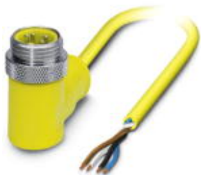
Sensor/actuator cable, 4-position, PVC, yellow, Plug angled 7/8"-16UNF, A-coded, on free cable end, cable length: 2 m
