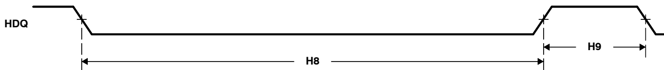
Figure 5–39. HDQ/1-Wire Break (Reset) Timing
