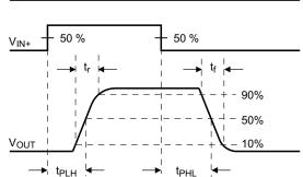
Figure 49. V<sub>OUT</sub> Propagation Delay, Non-inverting Configuration
