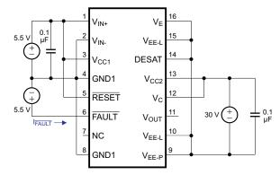
Figure 33. I<sub>FH</sub> Test Circuit
