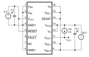
Figure 39. V<sub>OL</sub> Test Circuit
