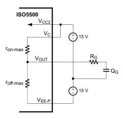
Figure 69. Simplified Output Model for Calculating Pol-WC
