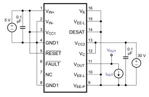
Figure 38. V<sub>OH</sub> Test Circuit
