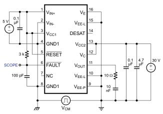
Figure 44. CMTI V<sub>FL</sub> Test Circuit
