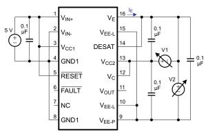
Figure 40. I<sub>EH</sub> Test Circuit
