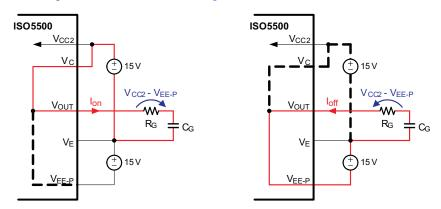
Figure 70. Simplified Gate Charge and Discharge Model
