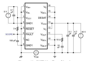
Figure 43. CMTI V<sub>FH</sub> Test Circuit
