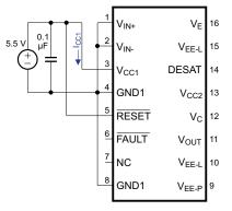
Figure 29. I<sub>CC1L</sub> Test Circuit
