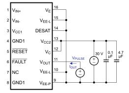
Figure 36.  $I_{OL}$  Test Circuit
