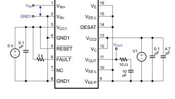
Figure 46. CMTI V<sub>OL</sub> Test Circuit
