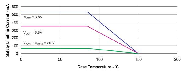
Figure 52. DW-16  $\theta_{JC}$  Thermal Derating Curve per DIN V VDE V 0884-10 (VDE V 0884-10)
