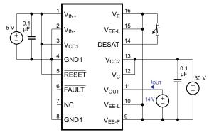
Figure 37.  $I_{OF}$  Test Circuit
