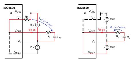
Figure 71. Reducing I<sub>ON-PK</sub> by Inserting Resistor R<sub>C</sub>
