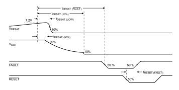
Figure 51. DESAT, V<sub>OUT</sub>, FAULT, RESET Delays
