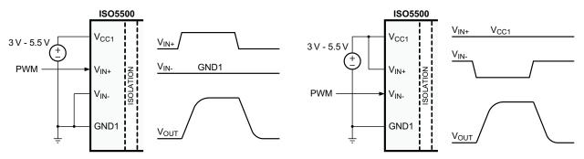
Figure 56. Non-inverting (left) and Inverting (right) Input Configurations
