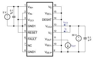
Figure 30.  $I_{CC2H}$ ,  $I_{CH}$  Test Circuit
