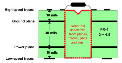
Figure 74. Recommended Layer Stack
