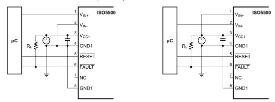
Figure 64. Local Shutdown and Reset for Noninverting (left) and Inverting Input Configuration (right)
