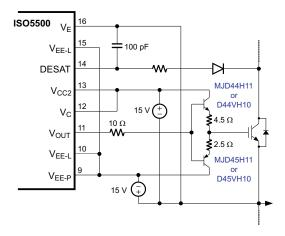
Figure 72. Current Buffer for Increased Drive Current
