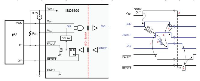
Figure 60. Fault Alarm Circuitry and Timing Sequence
