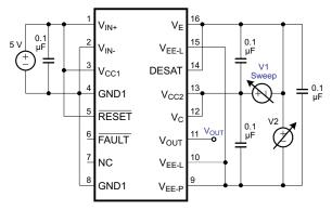
Figure 32. V<sub>IT(UVLO)</sub> Test Circuit
