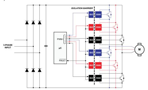
Figure 61. Typical Motor Drive Application
