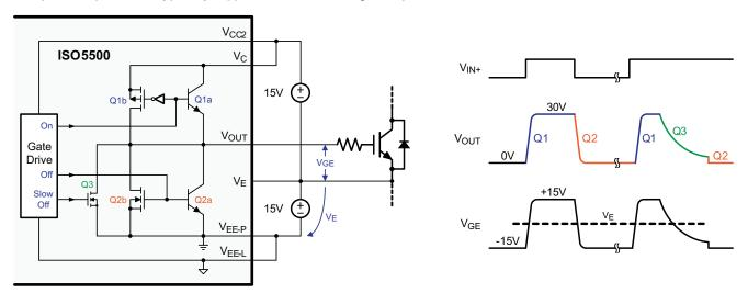
Figure 57. Output Stage Design and Timing
