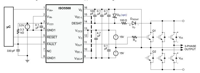
Figure 62. Recommended Application Circuit
