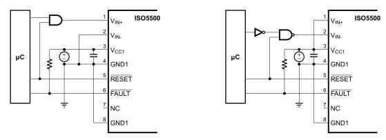
Figure 67. Auto Reset with Prior Gate-low Assertion for Non-inverting and Inverting Input Configuration
