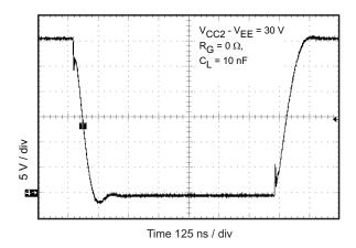
Figure 73. Output Waveform
