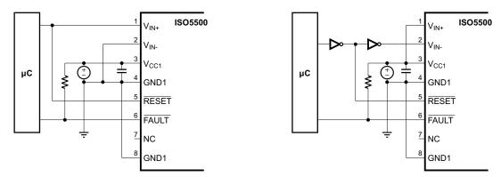
Figure 66. Auto Reset for Non-inverting and Inverting Input Configuration
