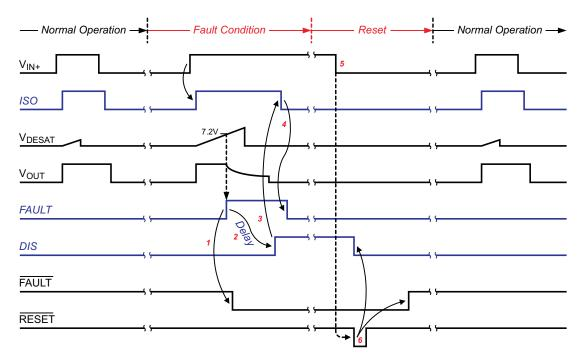
Figure 54. Complete Timing Diagram
