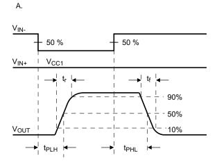
Figure 50. V<sub>OUT</sub> Propagation Delay, Inverting Configuration
