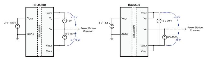
Figure 55. Power Supply Configurations
