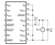
Figure 31.  $I_{CC2L}$ ,  $I_{CL}$  Test Circuit
