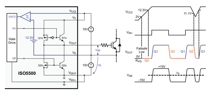
Figure 58. Undervoltage Lockout (UVLO) Function
