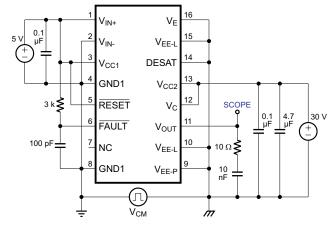
Figure 45. CMTI V<sub>OH</sub> Test Circuit
