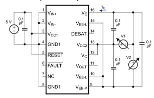
Figure 41. I<sub>EL</sub> Test Circuit
