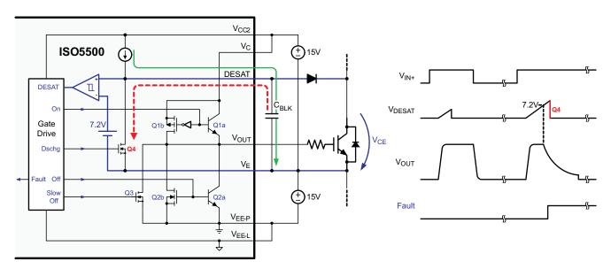
Figure 59. DESAT Fault Detection and Protection
