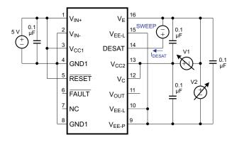
Figure 42.  $I_{CHG}$ ,  $I_{DSCHG}$ ,  $V_{DSTH}$  Test Circuit
