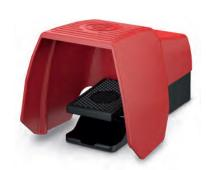
Standard OFF-ON Operation -Push pedal to change contact state. Release pedal to return to original state. With 2NC contact Emergency Stop Standard and Latching style with built in contactor can switch up to 16AMPS@400VAC for AC1 applications, with additional 3NO/1NC Contacts Analog Output Operation -As the pedal is depress, voltage or amperage (depending on model) is increase. Features an additional programmable PNP NO signaling contact that activates at a preset level.
