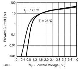
Fig. 4 - Max. Forward Current vs. Forward Voltage
