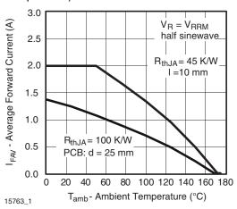
Fig. 3 - Max. Average Forward Current vs. Ambient Temperature
