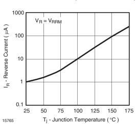
Fig. 2 - Max. Reverse Current vs. Junction Temperature
