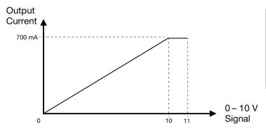
Dimming Resistor between "Dimming" and "SGND"
