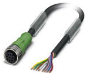
Sensor/actuator cable, 8-position, PUR halogen-free, black-gray RAL 7021, free cable end, on Socket straight M12, A-coded, cable length: 20 m
