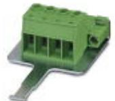
Plug component, Nominal current: 76 A, Rated voltage (III/2): 1000 V, Number of positions: 4, Pitch: 10.16 mm, Connection method: Screw connection with tension sleeve, Color: green, Contact surface: Silver
