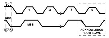
FIGURE 17. ACKNOWLEDGE ON THE I<sup>2</sup>C BUS
