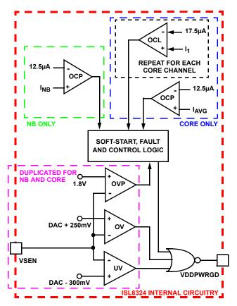
FIGURE 13. POWER-GOOD AND PROTECTION CIRCUITRY
