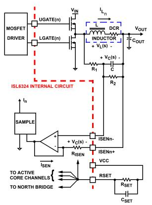
FIGURE 5. INDUCTOR DCR CURRENT SENSING CONFIGURATION
