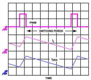
FIGURE 4. CONTINUOUS CURRENT SAMPLING
