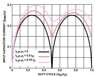
FIGURE 28. NORMALIZED INPUT-CAPACITOR RMS
