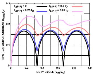
FIGURE 27. NORMALIZED INPUT-CAPACITOR RMS
