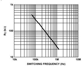
FIGURE 25. RT vs SWITCHING FREQUENCY
