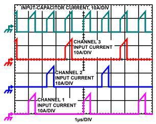
FIGURE 2. CHANNEL INPUT CURRENTS AND INPUT
