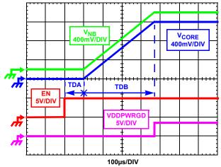
FIGURE 11. SOFT-START WAVEFORMS
