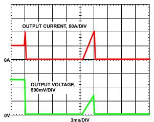
FIGURE 14. OVERCURRENT BEHAVIOR IN HICCUP MODE
