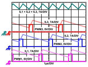
FIGURE 1. PWM AND INDUCTOR-CURRENT WAVEFORMS
