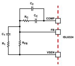
FIGURE 24. COMPENSATION CIRCUIT WITHOUT LOAD-LINE REGULATION
