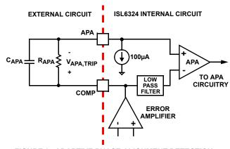
FIGURE 3. ADAPTIVE PHASE ALIGNMENT DETECTION
