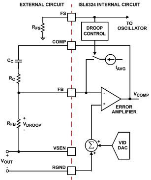
FIGURE 8. OUTPUT VOLTAGE AND LOAD-LINE REGULATION
