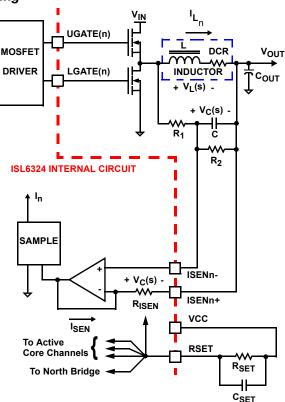
FIGURE 21. DCR SENSING CONFIGURATION
