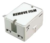
One of the major considerations when using a SSR is properly managing the heat that is generated when switching currents higher than about 5 amps. In this scenario one must mount the base plate of the SSR onto a good heat conductor, typically aluminum; along with utilizing a good thermal transfer medium such as thermal grease or heat transfer pad. Magnecraft's thermal pad eliminates the need for messy thermal grease and simplifies installation with a simple peel-and-stick solution.
