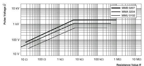
10 pulses at 1 minute intervals; for permissible resistance change  $\pm$  (0.5 % R + 0.05  $\Omega$ )
