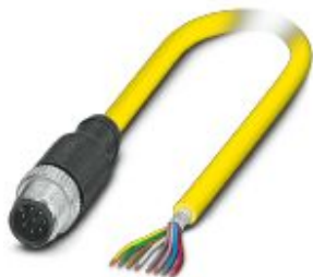
Sensor/actuator cable, 8-position, PVC, yellow, shielded, Plug straight M12 SPEEDCON, coding: A, on free cable end, cable length: 5 m
