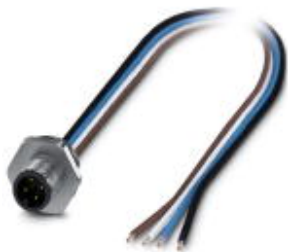
Flush-type connector, Universal, 5-position, Plug, M12, A-coded, Front mounting, M16 x 1.5, Individual wires, cable length: 0.5 m
