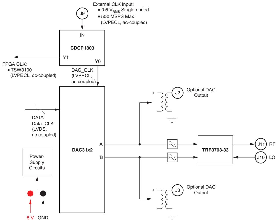
Figure 1. DAC31x2EVM Block Diagram
