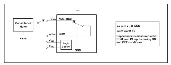
Figure 15. Capacitance (C<sub>I</sub>, C<sub>COM(ON)</sub>, C<sub>NO(OFF)</sub>, C<sub>COM(OFF)</sub>, C<sub>NO(ON)</sub>)
