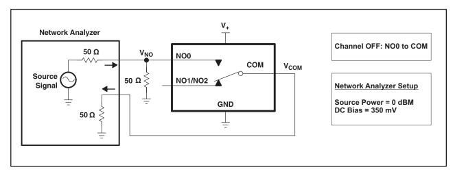
Figure 19. OFF Isolation (O<sub>ISO</sub>)
