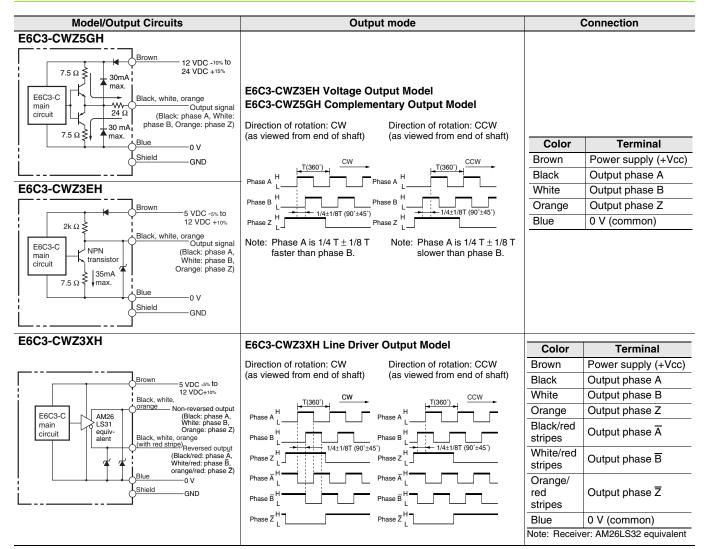
Note: 1. The shielded cable outer core (shield) is not connected to the inner area or to the case.
