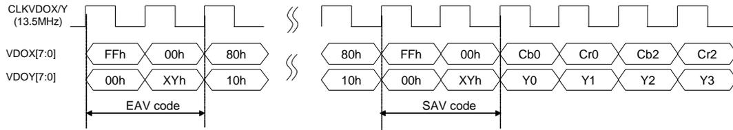
FIGURE 66 TIMING DIAGRAM OF SINGLE OUTPUT MODE FOR 601 INTERFACE
