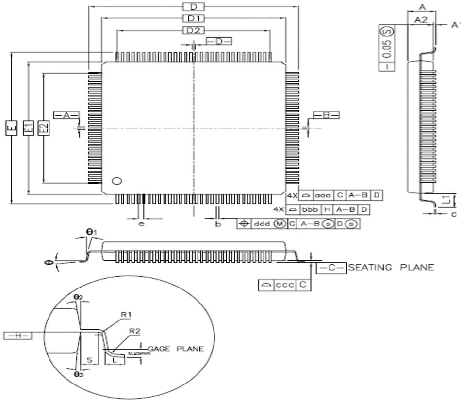
CONTROL DIMENSIONS ARE IN MILLIMETERS.
