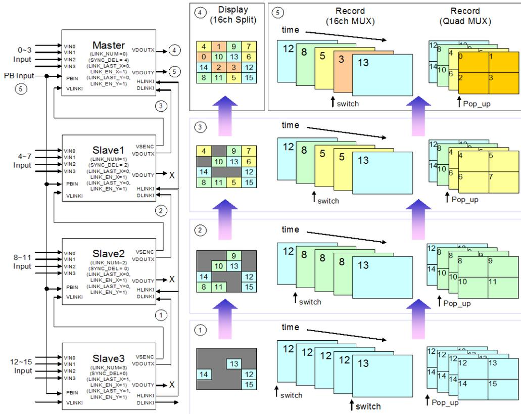
**FIGURE 48 THE CASCADE CONNECTION FOR 120 CIF/SEC RECORD MODE**
