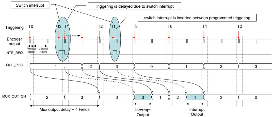
FIGURE 26 THE INTERRUPTED SWITCHING SEQUENCE WHEN QUE\_SIZE = 3, QUE\_PERIOD = 1
