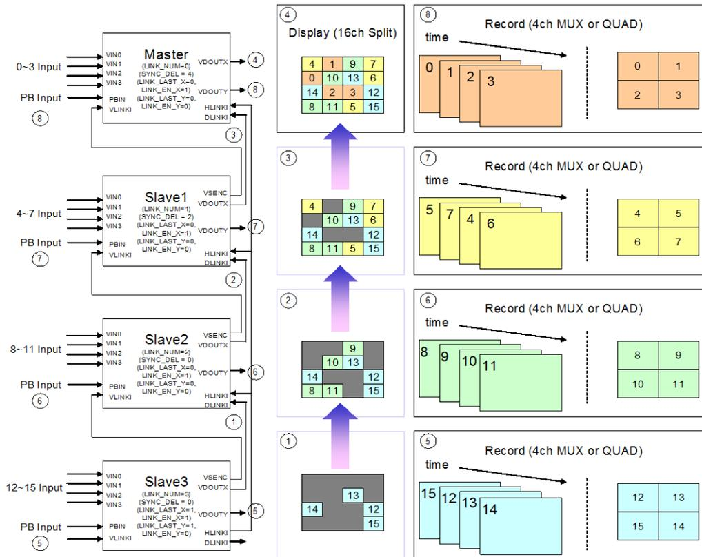
**FIGURE 50 THE CASCADE CONNECTION FOR 480 CIF/SEC RECORD MODE**
