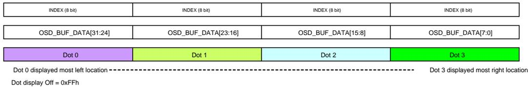
OSD\_BUF\_DATA for display path in 64 color mode Compatible with TW2835
