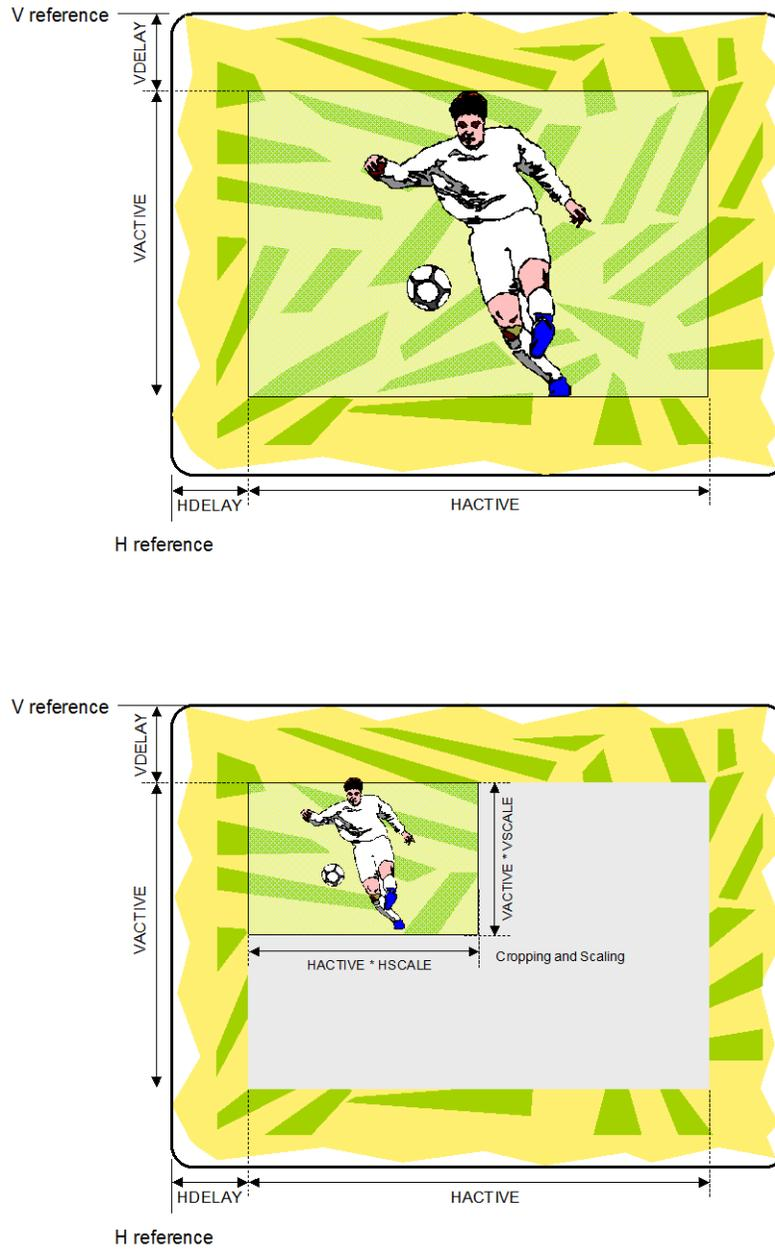
**FIGURE 12 THE EFFECT OF CROPPING AND SCALING**
