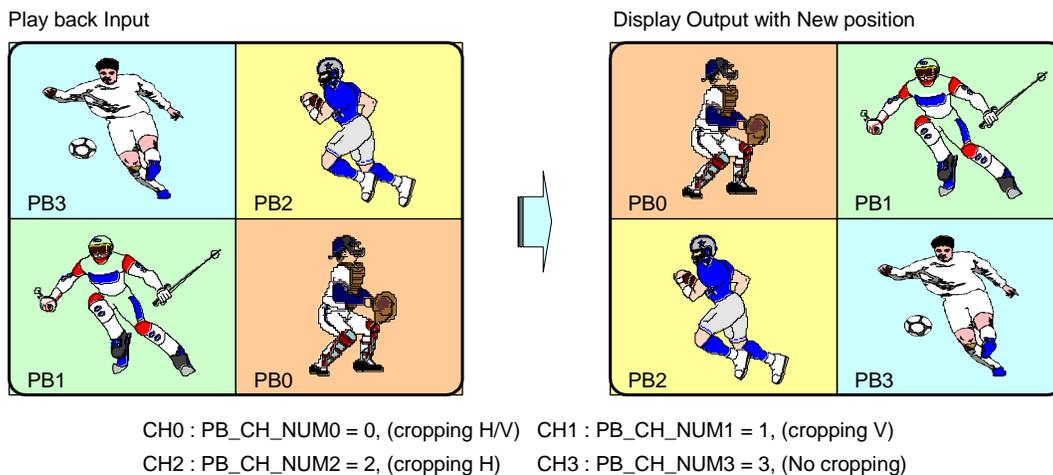
**FIGURE 13 THE EFFECT OF AUTO CROPPING FUNCTION**
