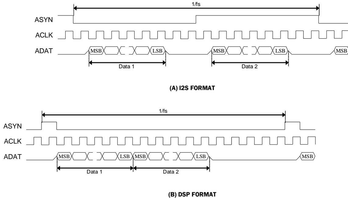
FIGURE 73 TIMING CHART OF SERIAL AUDIO INTERFACE
