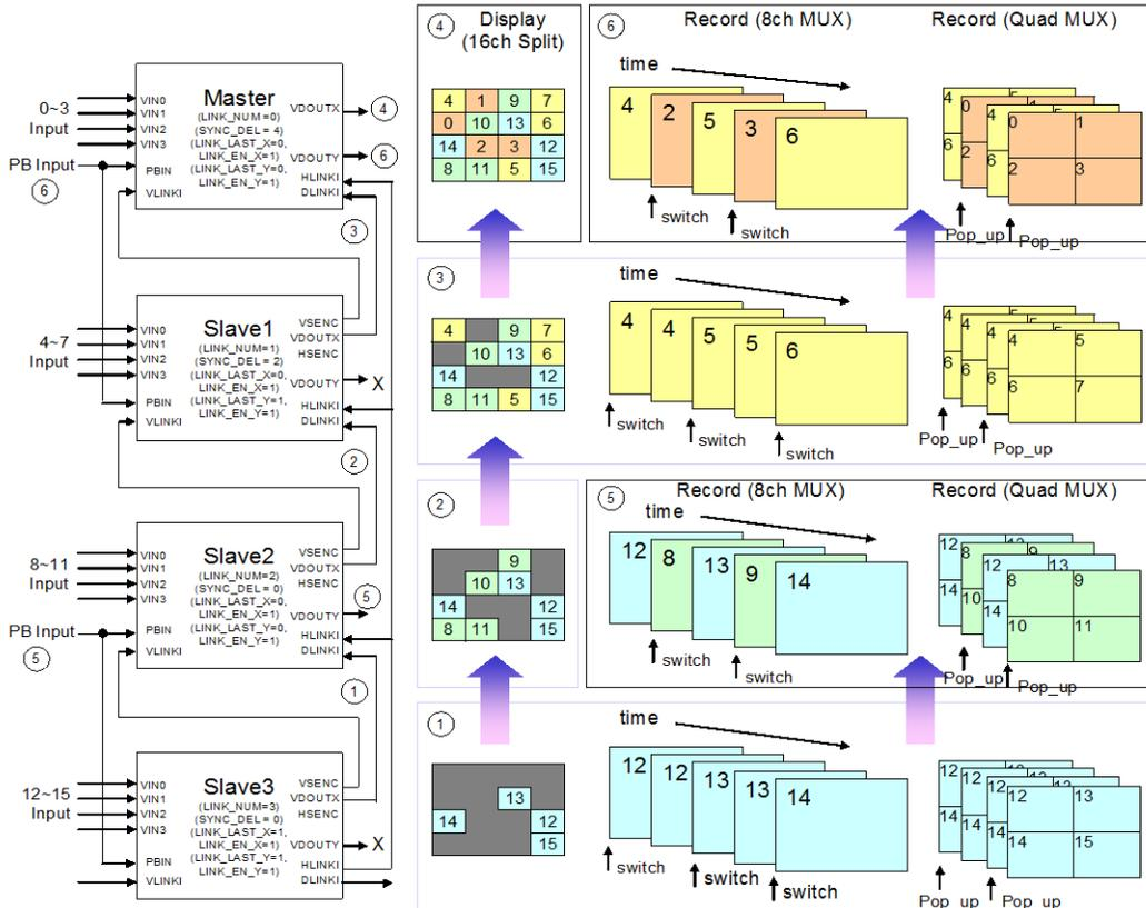
FIGURE 49 THE CASCADE CONNECTION FOR 240 CIF/SEC RECORD MODE
