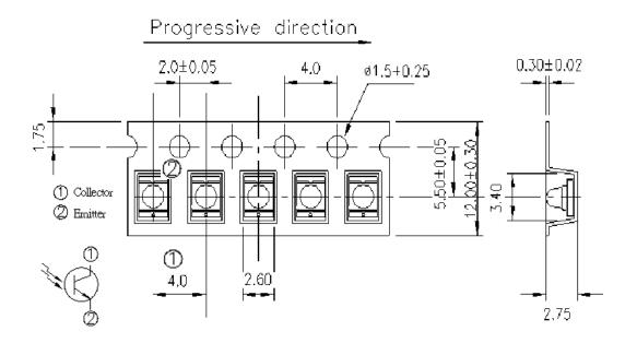
**Note:** The tolerances unless mentioned are ±0.1, unit=mm.
