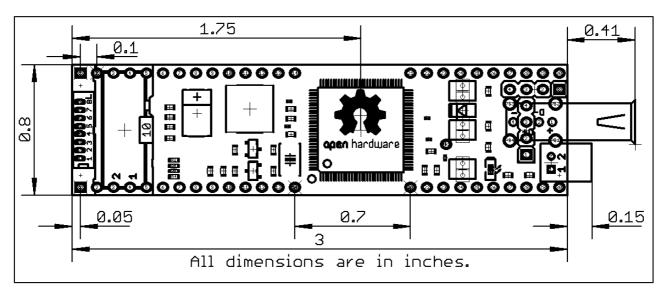
Note that the iMX233-OLinuXino-NANO board has a 6-layer PCB. The three highest elements on the board in order from the tallest to the shortest are: vertical USB HOST – 16.2mm (0.640") over the pcb; UEXT connector – 13.6mm (0.525"); U\_DEBUG pins – 12.0mm(0.464").
