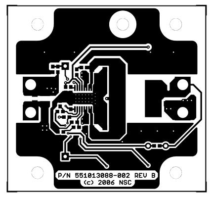
Figure 6. Component Side
