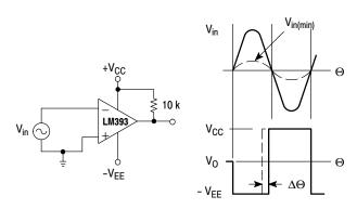
$V_{in(min)} \approx 0.4 \text{ V}$  peak for 1% phase distortion ( $\Delta\Theta$ ).
