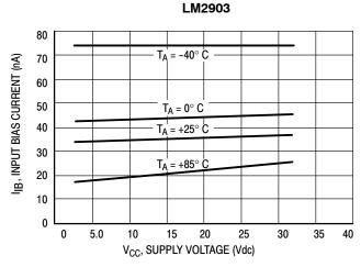
Figure 3. Input Bias Current versus Power Supply Voltage
