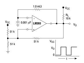
Figure 10. Free-Running Square-Wave Oscillator
