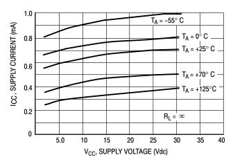
Figure 6. Power Supply Current versus Power Supply Voltage
