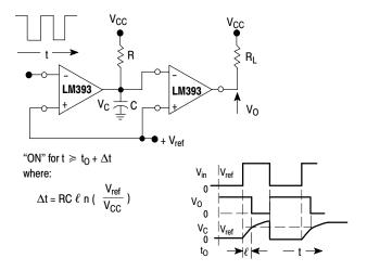
Figure 11. Time Delay Generator
