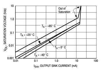
Figure 5. Output Saturation Voltage versus Output Sink Current
