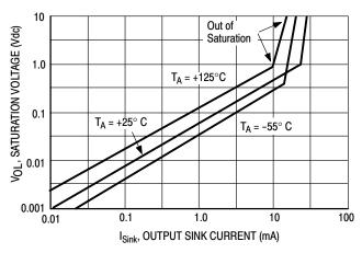
Figure 4. Output Saturation Voltage versus Output Sink Current
