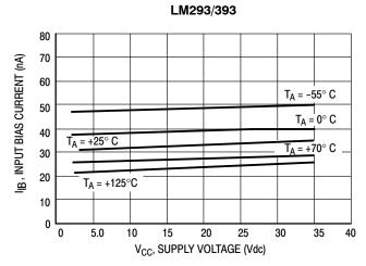
Figure 2. Input Bias Current versus Power Supply Voltage
