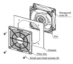
Replacement filters can be replaced by taking off the front part of the filter kit. There is no need to remove the screws.
