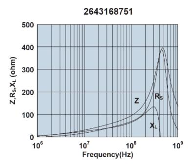
Impedance, reactance, and resistance vs. frequency.
