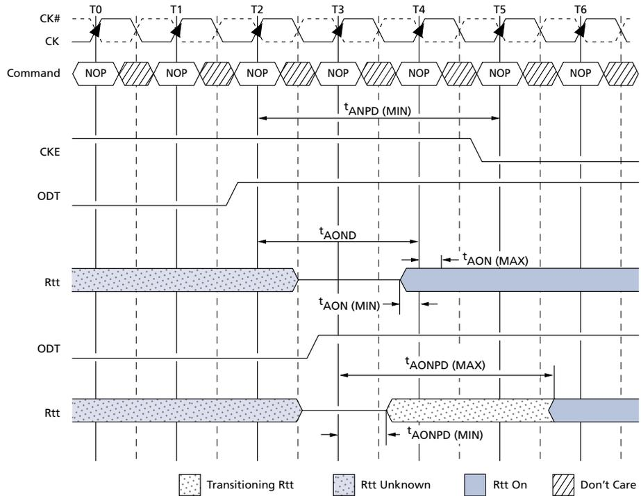
Figure 89: ODT Turn-Off Timing When Exiting Power-Down Mode
