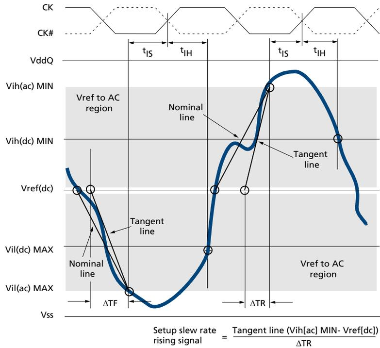
Figure 28: Nominal Slew Rate for  $t_{IH}$
