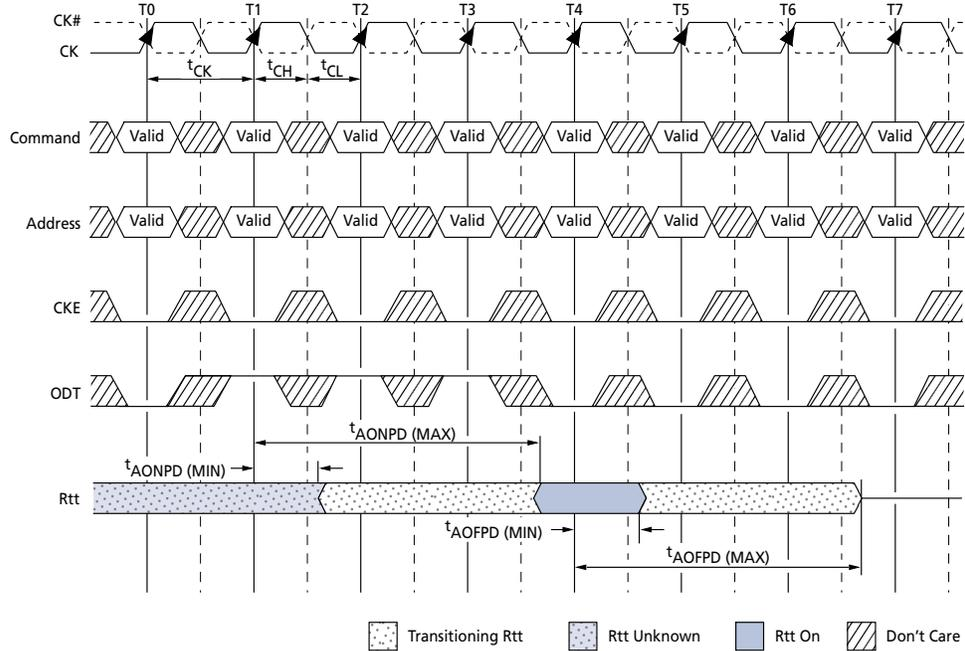
Figure 87: ODT Turn-Off Timings When Entering Power-Down Mode
