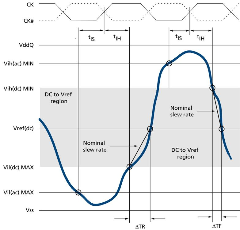
**Figure 29: Tangent Line for t<sub>IH</sub>**
