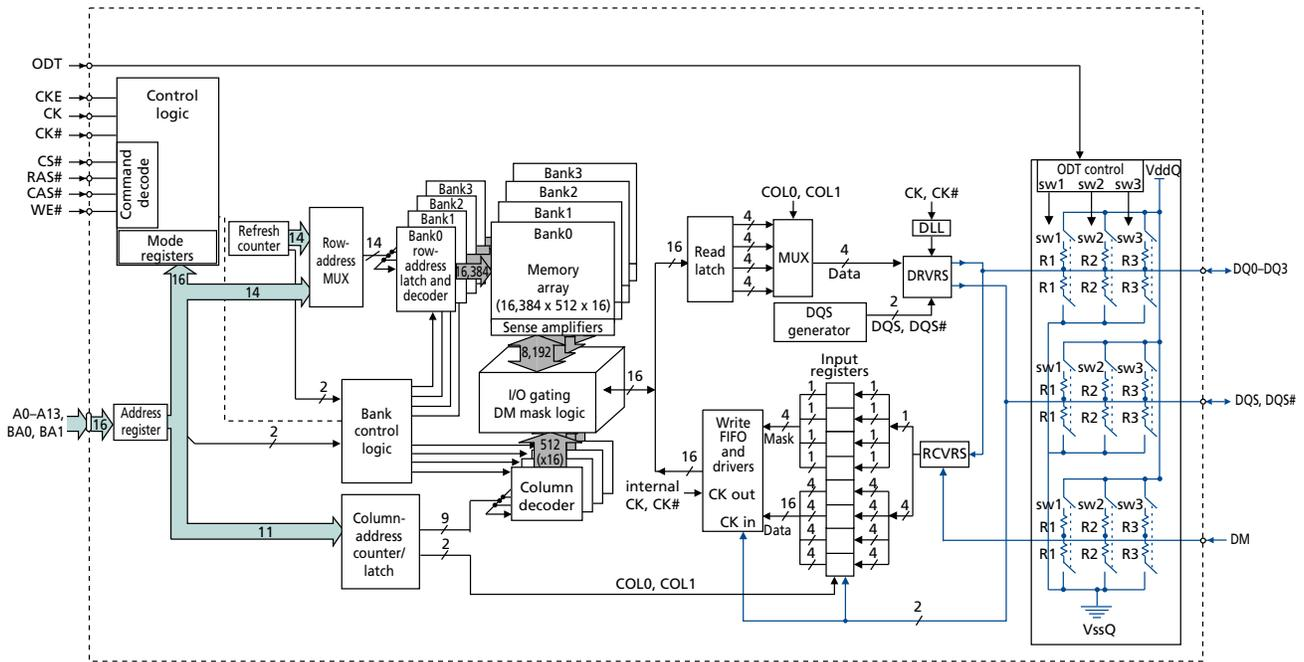
**Figure 4: 64 Meg x 8 Functional Block Diagram**
