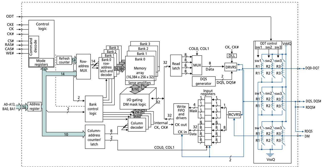
**Figure 5: 32 Meg x 16 Functional Block Diagram**
