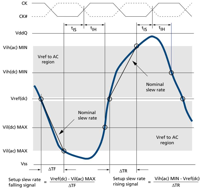
Figure 27: Tangent Line for  $t_{1S}$
