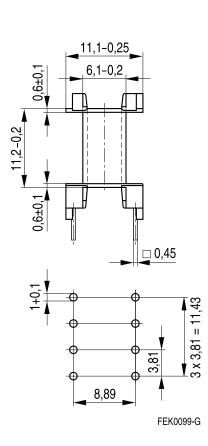
Hole arrangement View in mounting direction
