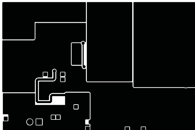
Figure 41. TPS40200EVM-001 Bottom Copper (X-Ray View from Top)
