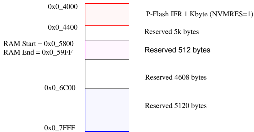
Figure 25-3. Memory Controller Resource Memory Map (NVMRES=1)
