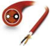
Highly flexible POF round cable (IP20 heads only) for use in drag chains. Individual elements made from extremely wear-resistant polyamide (PE). The cable is halogen-free, ozone and UV resistant, and has a rugged polyurethane (PUR) outer sheath.
