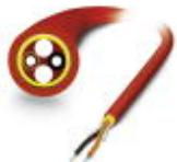
Rugged POF installation cable (IP20 heads only) for fixed installation in the inner area. Individual elements made from extremely wear-resistant polyamide (PE). Halogen-free, ozone and UV resistant with a reinforced polyurethane (PUR) outer sheath.
