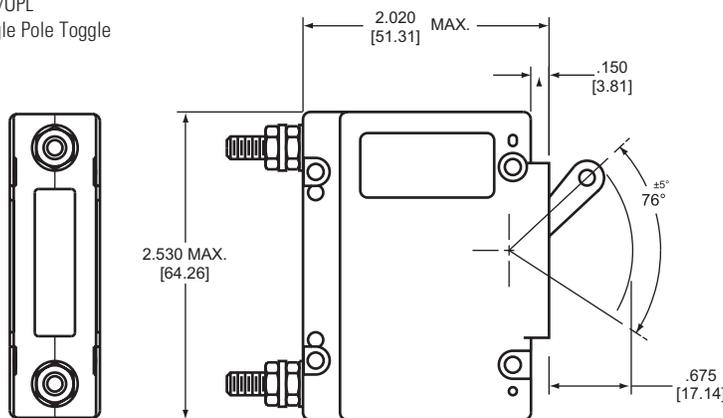
Note: Tolerance  $\pm .015$  [.38] unless noted. Dimensions in brackets [ ] are millimeters.
