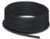
Master cable for sensor/actuator boxes, without PE conductor, unshielded, material PUR/PVC, 6-pos., 4 x 0.34 mm<sup>2</sup> and 2 x 0.75 mm<sup>2</sup>, length: 50 m
