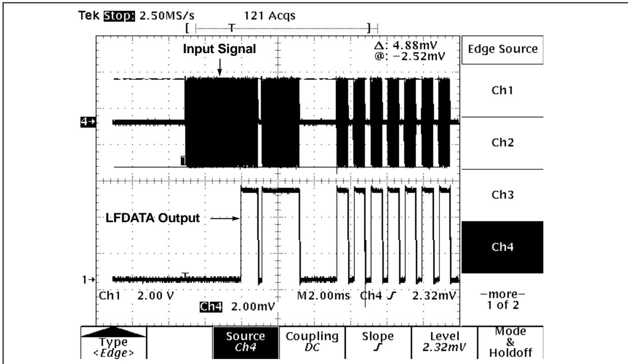
**Case II. When Output Enable Filter is enabled:** Demodulated output is available only if the incoming signal meets the enable filter timing criteria that is defined in the Configuration Register 0 (Register 11-1). If the criteria is met, the output is available after the low timing (TOEL) of the Enable Filter. Figure 11-11 and Figure 11-12 shows examples of demodulated output when the Output Enable Filter is enabled.
