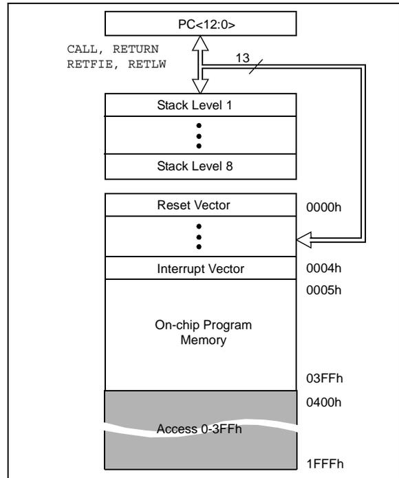
FIGURE 2-2: PROGRAM MEMORY MAP AND STACK OF THE PIC16F636/639
