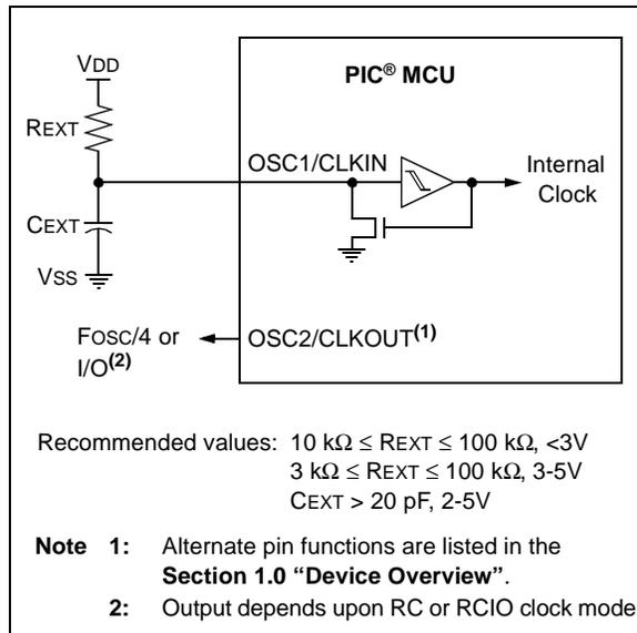
In RCIO mode, the RC circuit is connected to OSC1. OSC2 becomes an additional general purpose I/O pin.
