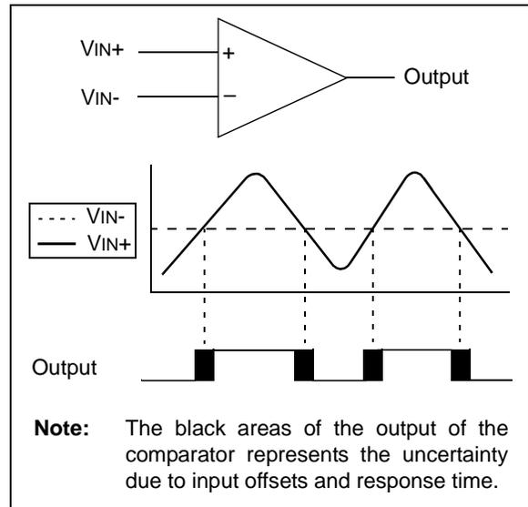
**FIGURE 7-2: COMPARATOR OUTPUT BLOCK DIAGRAM (PIC12F635)**
