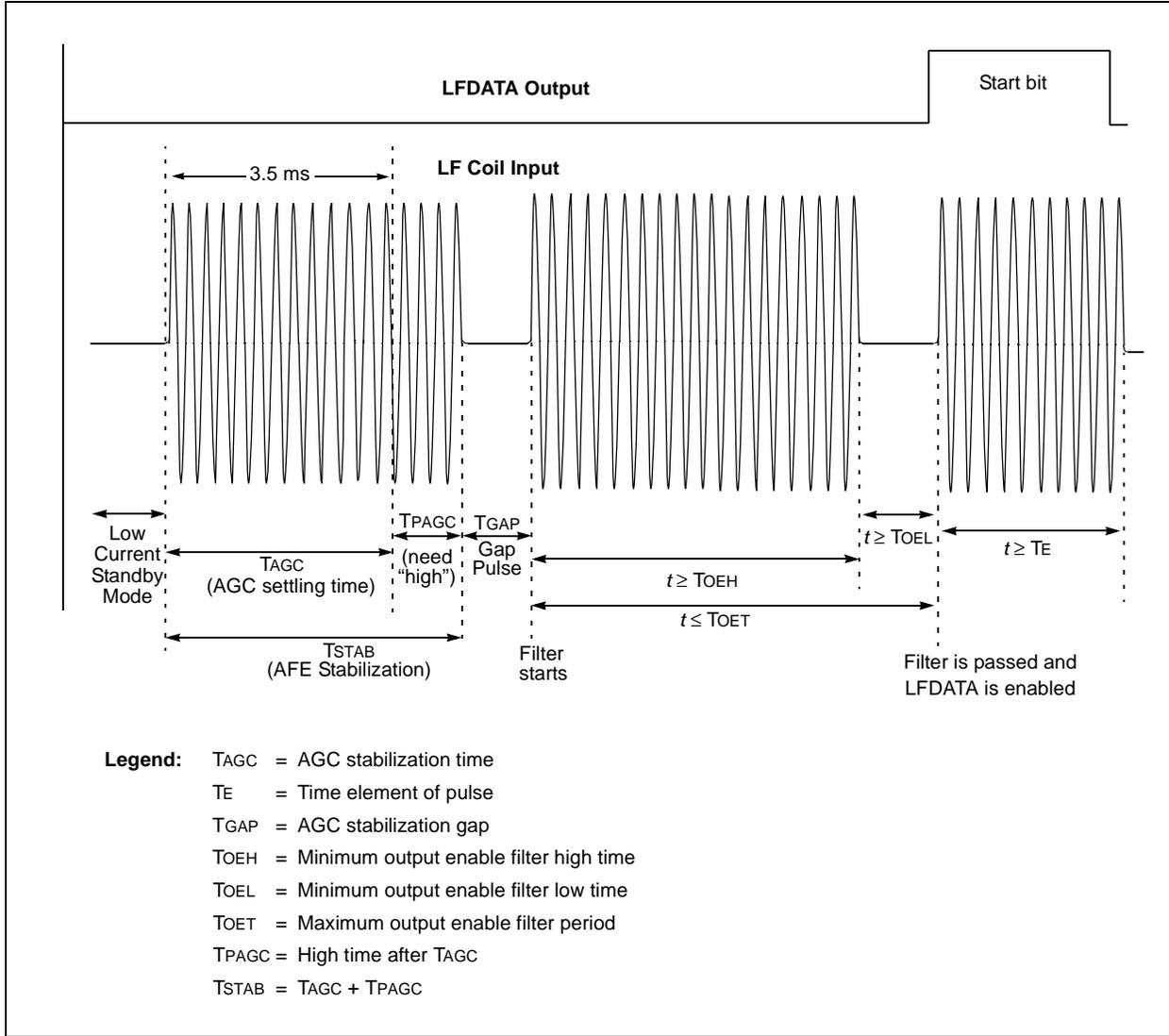
**TABLE 11-1: TYPICAL OUTPUT ENABLE FILTER TIMING**
