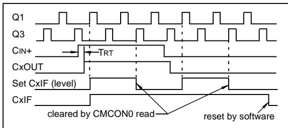
**Note 1:** If a change in the CMCON0 register (CxOUT) should occur when a read operation is being executed (start of the Q2 cycle), then the CxIF of the PIR1 register interrupt flag may not get set.
