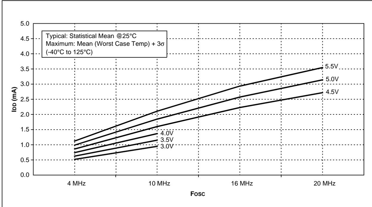
**FIGURE 16-5: TYPICAL  $I_{DD}$  vs.  $V_{DD}$  OVER  $F_{osc}$  (XT MODE)**
