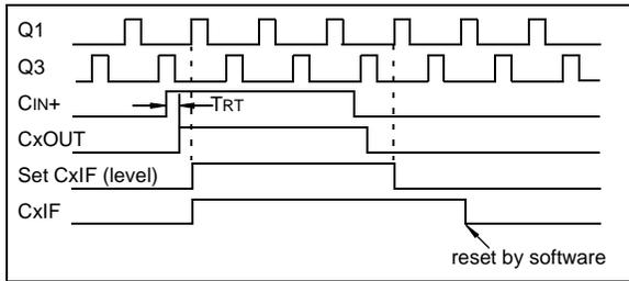
**FIGURE 7-9: COMPARATOR INTERRUPT TIMING WITH CMCON0 READ**
