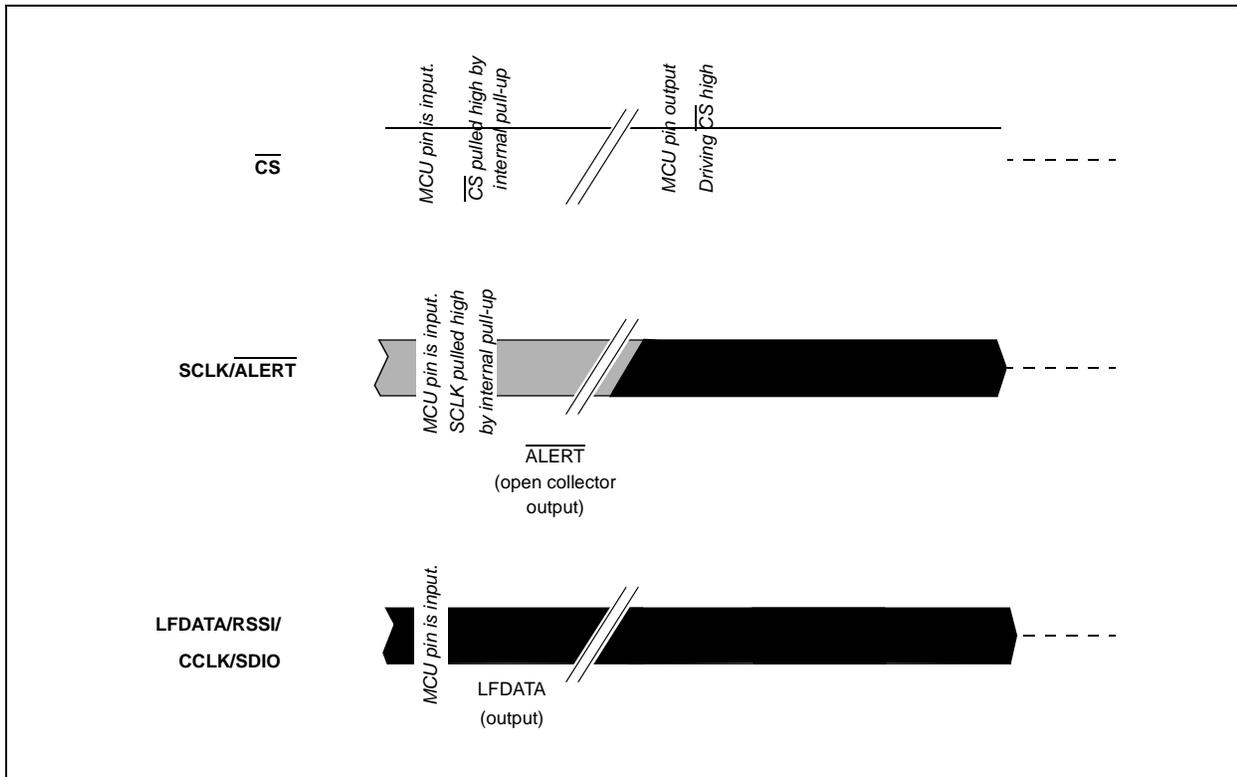
**FIGURE 11-17: SPI WRITE SEQUENCE**
