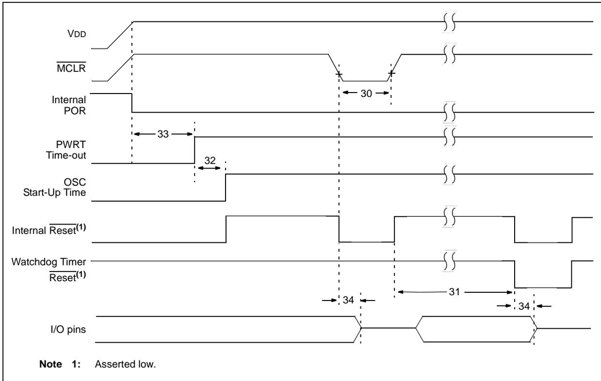
**FIGURE 15-8: BROWN-OUT RESET TIMING AND CHARACTERISTICS**
