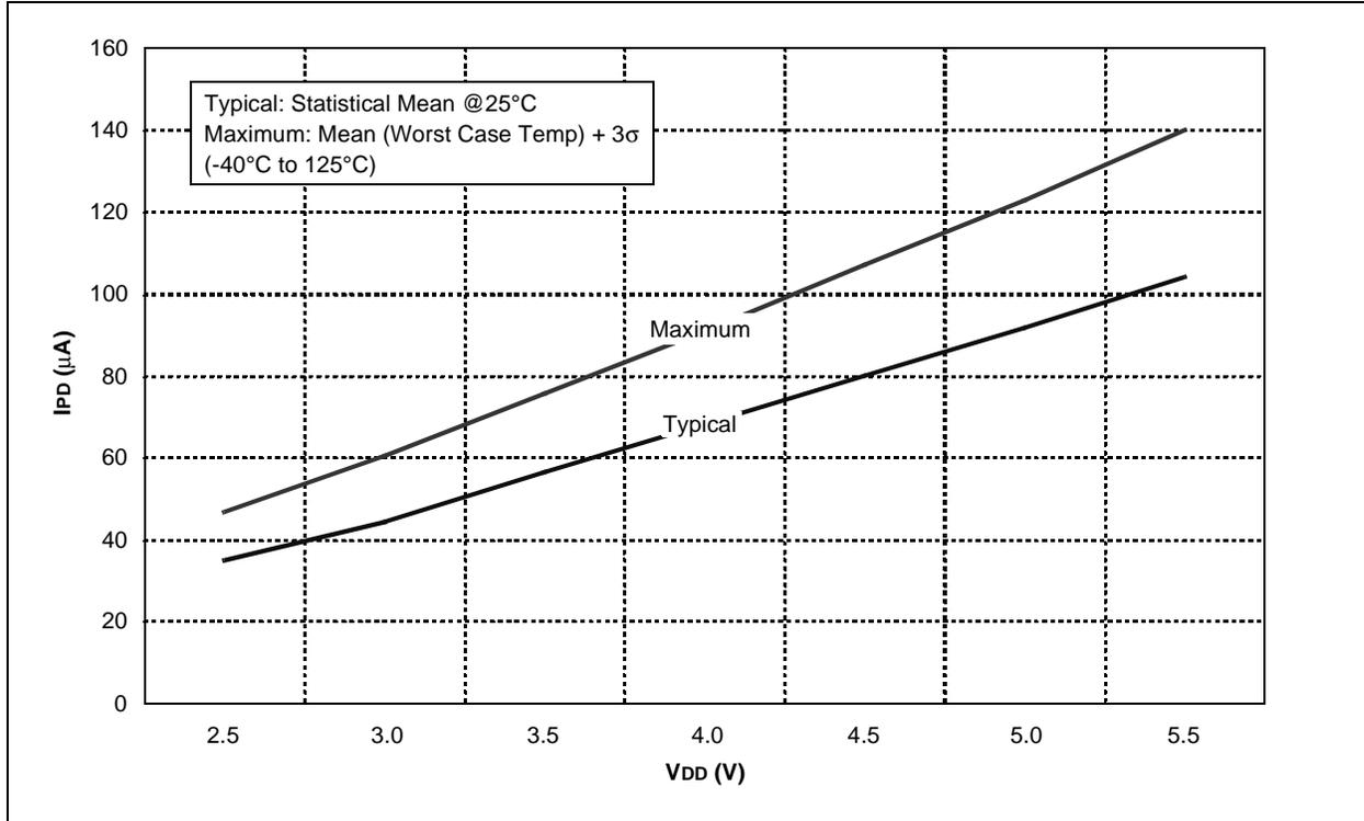
**FIGURE 16-17: TYPICAL WDT IPD vs. VDD OVER TEMPERATURE**
