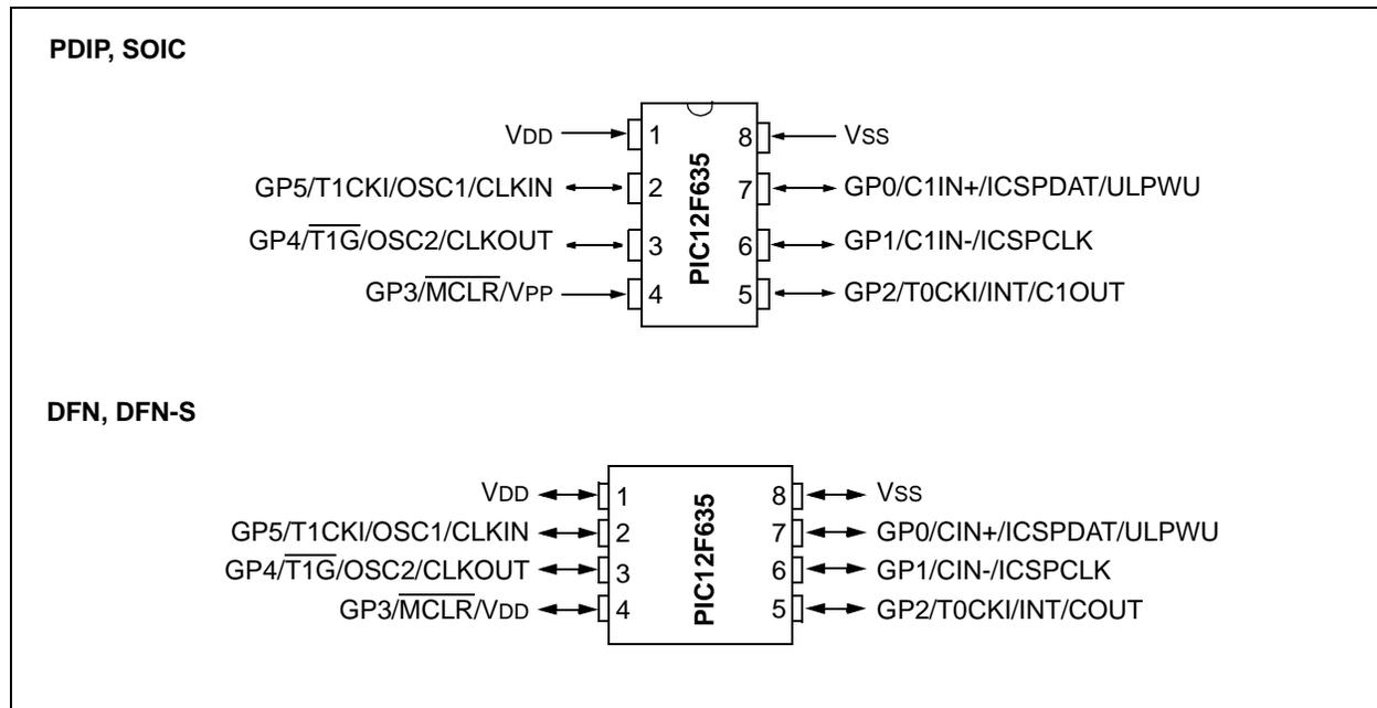
**TABLE 1: 8-PIN SUMMARY (PDIP, SOIC, DFN, DFN-S)**
