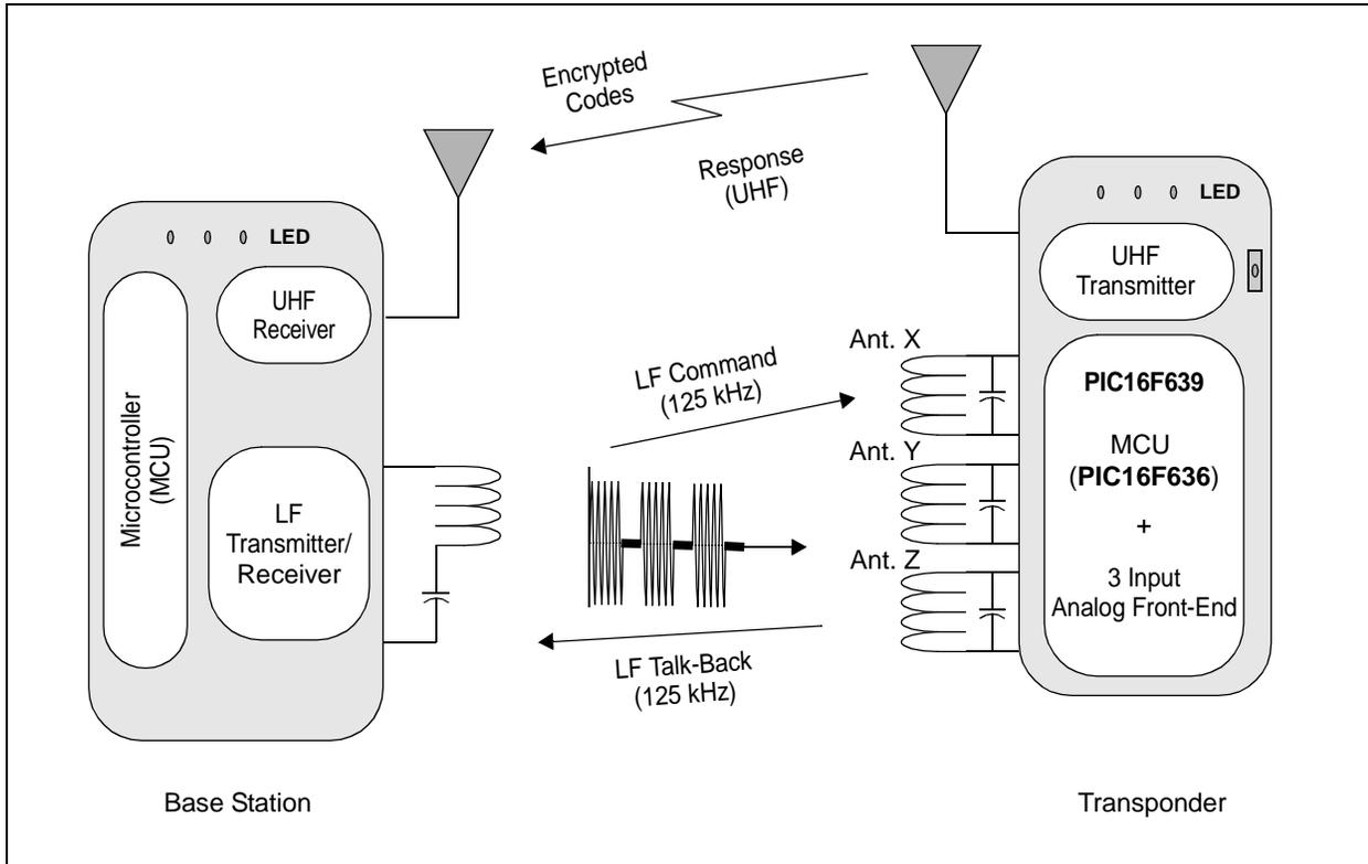
**FIGURE 11-4: PASSIVE KEYLESS ENTRY (PKE) TRANSPONDER CONFIGURATION EXAMPLE**
