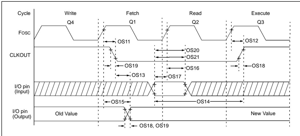
**TABLE 15-3: CLKOUT AND I/O TIMING PARAMETERS**
