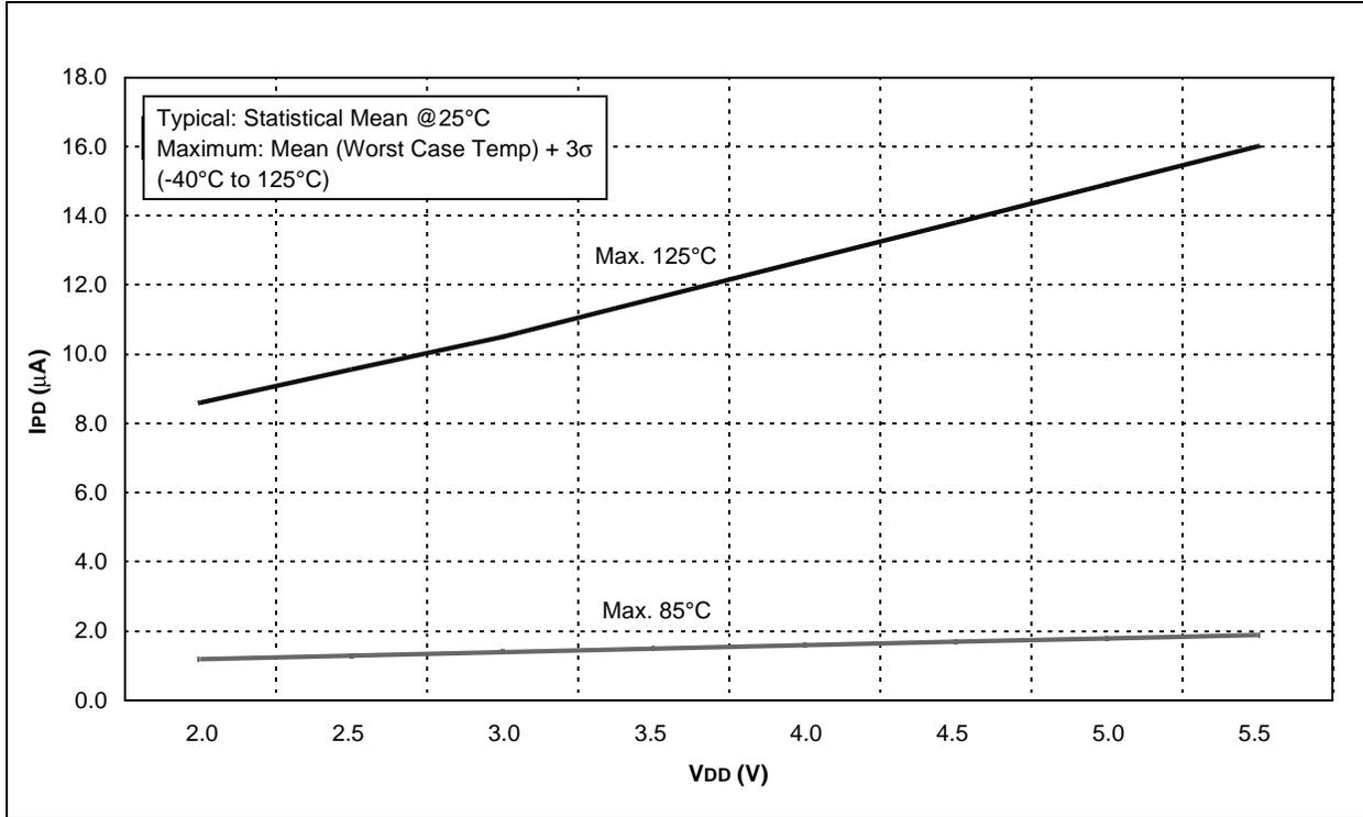
FIGURE 16-15: COMPARATOR IPD vs. VDD (BOTH COMPARATORS ENABLED)
