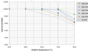
Fig. 3: Available load current vs. ambient air temperature and airflow rates for UIE48T10120 converter w/o baseplate mounted vertically with air flowing from pin 3 to pin 1, MOSFET temperature ≤ 125°C, Vin=24V
