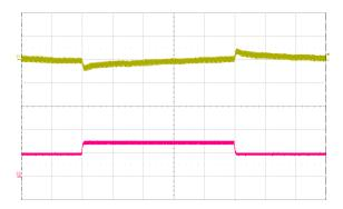
Fig. 13: Output voltage ripple (50 mV/div.) at full rated load current into a resistive load with Co = 10 μF tantalum + 1 μF ceramic and Vin = 48 V. Time scale: 2 μs/div.
