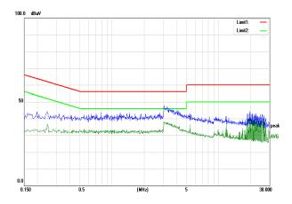
Fig. 20: Vin- Peak Detector EMI waveform
